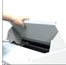
Rear safety cover Closing it initiates the slicing process and it opens automatically when slicing is complete.
